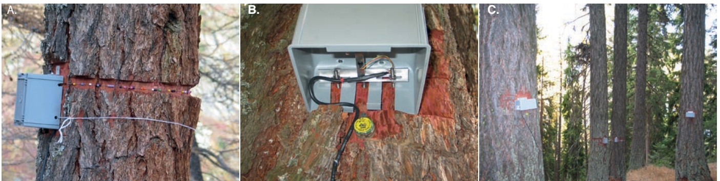
Figure 1.3. Pictures of a band or circumference dendrometer (A), a point or radial dendrometer (B) and installed dendrometers at a site used in my dissertation (C).
