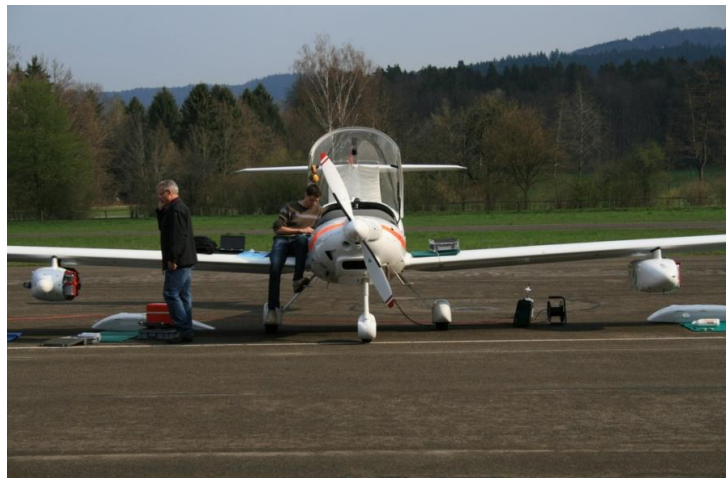
Figure 4: Preparing Metair Dimona for a research flight on 19 April 2011. The two underwing pods carry the measurement devices to collect volcanic data (picture: Metair).
