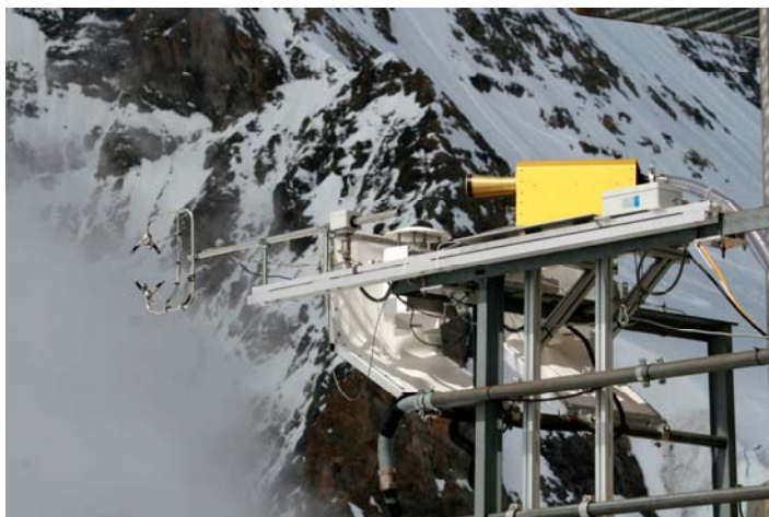
Fig. 3.4: Measurement setup from June 14 to July 19 of fog monitor and ultrasonic anemometer.
