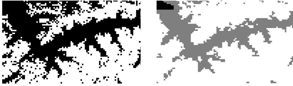
Figure 5.14: Resampled Landsat 5 TM snow map (left) and corresponding N14-AVHRR snow mask (right) showing the Rhone Valley at Martigny, Switzerland on May 3th, 1995. Both at a horizontal resolution of 1.1km. Snow pixels in white, snowfree pixels in black (left) or grey (right). Right black pixels correspond to invalid/cloud pixels. Landsat shows a much patchier snow map, even though the difference to the right AVHRR image is much smaller than in Figure 5.13 since both have same resolutions after the resampling of the Landsat snow mask.
