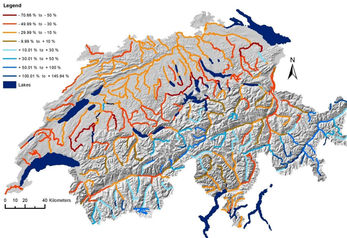
Figure 9 The percentage change in Q347 from the reference period to the 2085 period.
