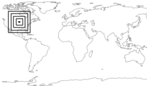
Figure 3: Visualization of the spatial dimension of different MW sizes. The central point corresponds to the initial MW centered grid cell. The first window visible is the 5x5 MW, then 7x7, 9x9 and 11x11.
