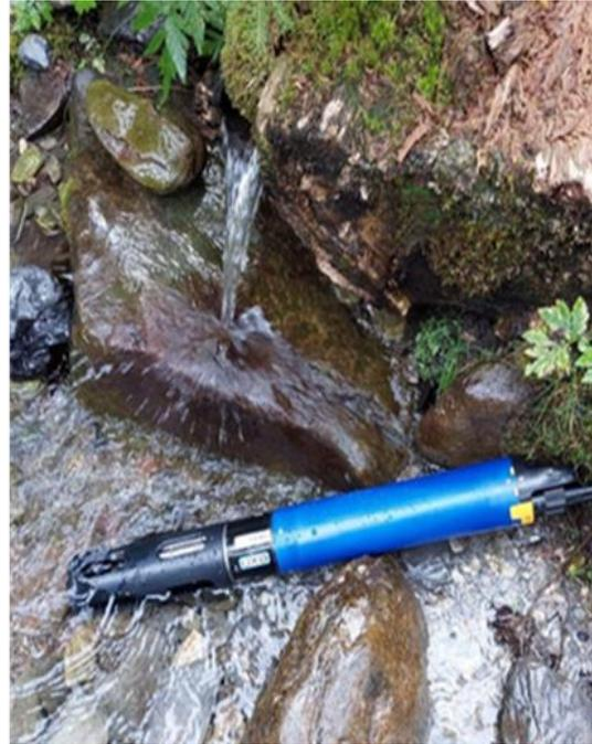
The EXO2 Sonde (EXO2 Multiparameter Sonde; YSI, Yellow Springs, United States) measures several water quality variables simultaneously and records the values over a predefined time period after having situated it into the water.
