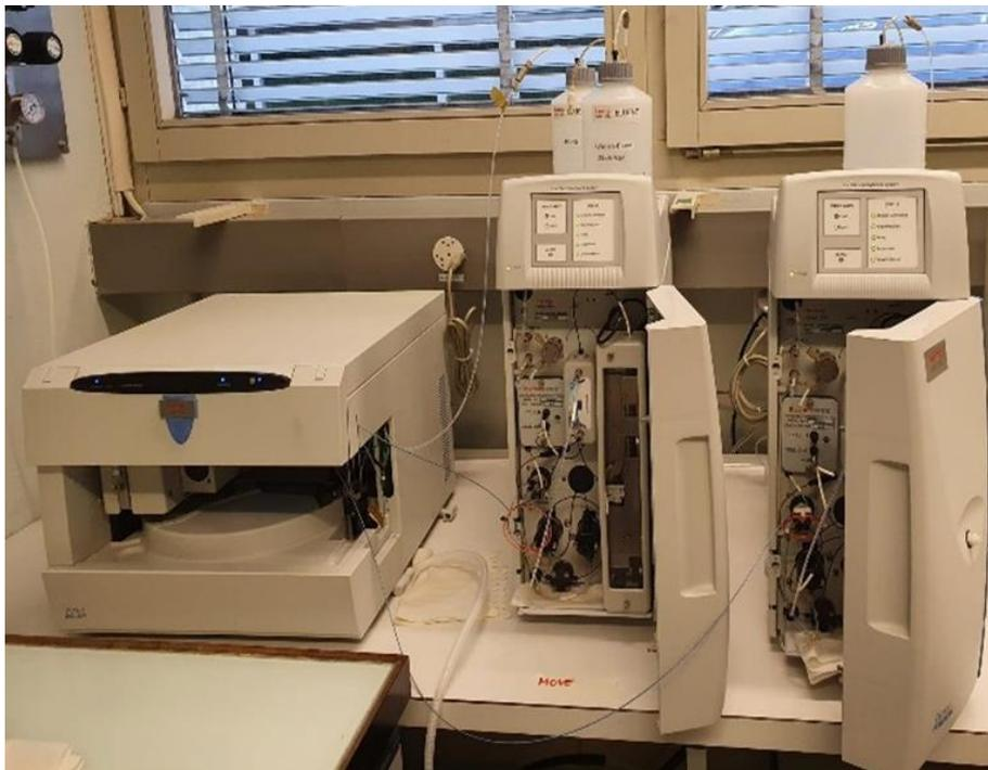
The concentration of a series of ions is determined by the ion chromatography machine (Dionex Aquion Ion Chromatography System; Thermo Fisher Scientific, Waltham, United States) in the lab at the Institute of Geography at the University of Bern.
