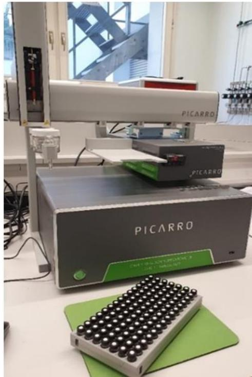
The L2140-I Isotope and Gas Concentration Analyzer (Picarro, Inc.; Santa Clara, California, USA) was used to determine the isotopic composition of water samples in the lab at the Institute of Geography at the University of Bern.
