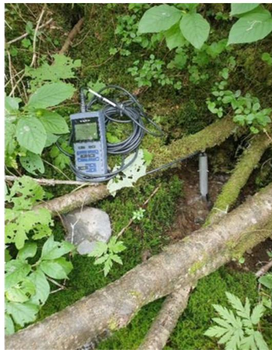
The pH value was measured by a pH-meter (WTW pH330i; Xylem Inc., Washington DC, United States) (left) and the temperature as well as the electrical conductivity by the WTW Portable Conductivity meter (Profiline Cond 3310; Xylem Inc., Washington DC, United States) (right).
