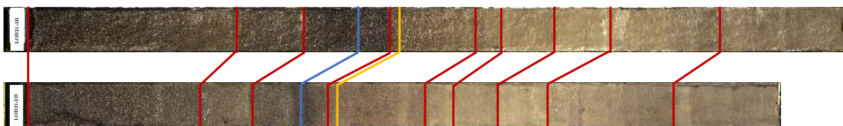
Fig. 20: Correlation of the master core LOB21-2 to core LOB21-3 used for PPP analysis. Visually correlated features are shown in red, blue denotes a feature identified from RABD_{615} , orange a feature correlated from R_{570}/R_{630} .
