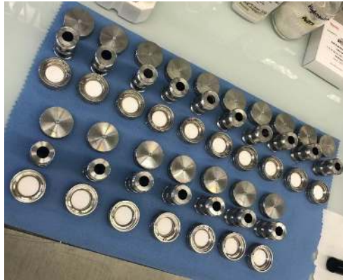
Figure 7. ASE assembly for sediment extraction with cell body and corresponding bottom and top covers. A big cellulose filter is placed in the bottom of the cell before closing.
