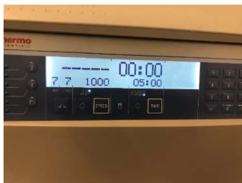
Figure 8. Centrifuge settings for the clean-up of sediment extracts
