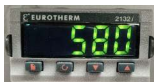
Figure 4: Over-temperature limiter setting for LOI 550
