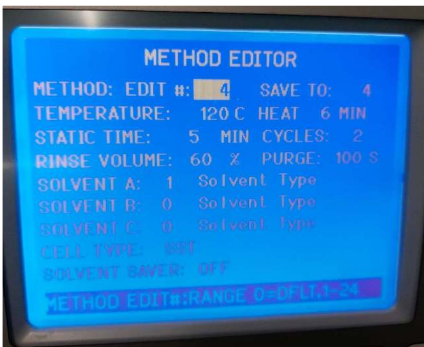
Figure 9. Method 4 shown in instrument. Method 4 uses 70:30 70:30 Acetone:1% phosphoric acid (%v/v)
