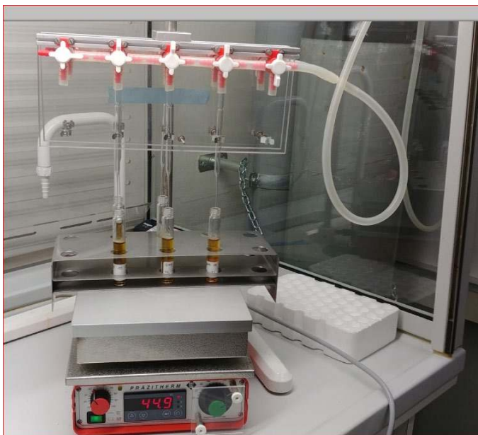
Figure 12. Nitrogen try set up for the evaporation of sediment extract.
