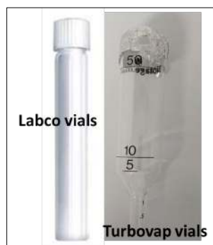
Figure 2. Labco and Turbovap vials needed for the evaporation and clean-up of sediment extracts
