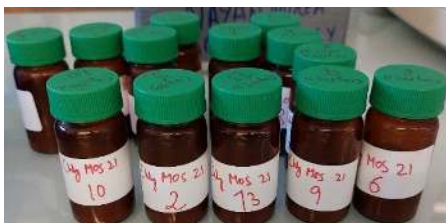
Figure 1. 20 ml glass containers for weighting and spiking of sediment samples
