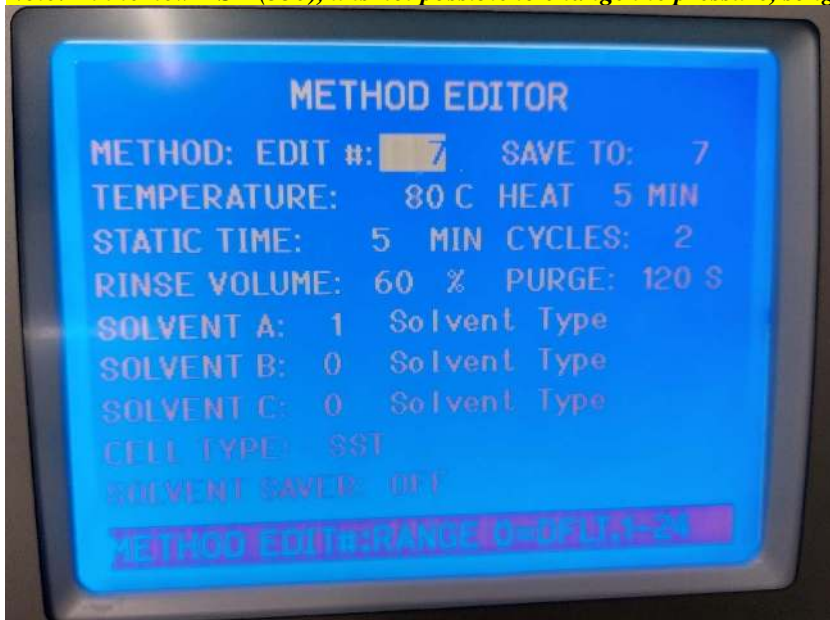
Figure 8. Method 7 as shown in instrument. Method 7 uses 70:30 Ethyl acetate: acetone (%v/v)
