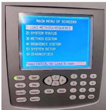
Figure 4. ASE 350 control panel. Press "tray" to unlock the collection and cell tray
