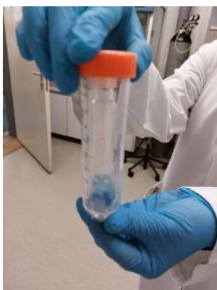
Figure 9. Labco vial inside of a Falcon tube use to protect the glass vial and extract.
