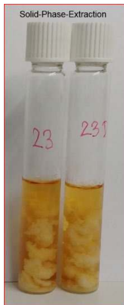
Figure 11. Addition of Kit 2 to sediment extracts for dSPE
