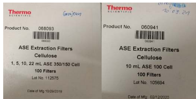
Figure 4. Big (left) and small (right) cellulose filters needed for the extraction of sediment samples
