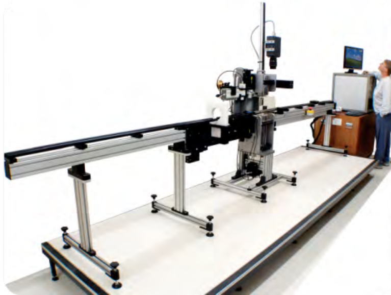
Fig. 3.2 A Geotek Multi-Sensor Core Logger (Geotek, n.d)
