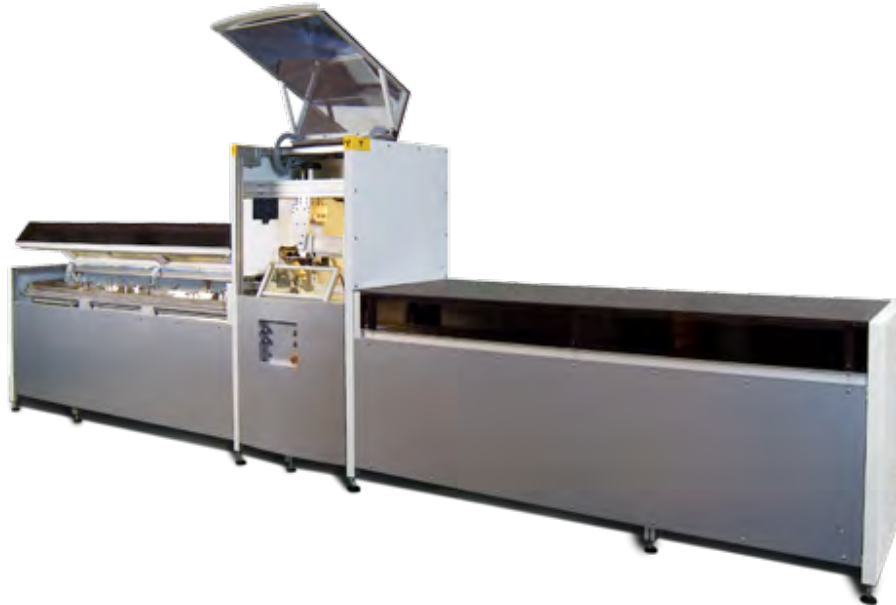
Fig. 3.3 An ITRAX XRF Core scanner (Cox Analytical System, n.d)
