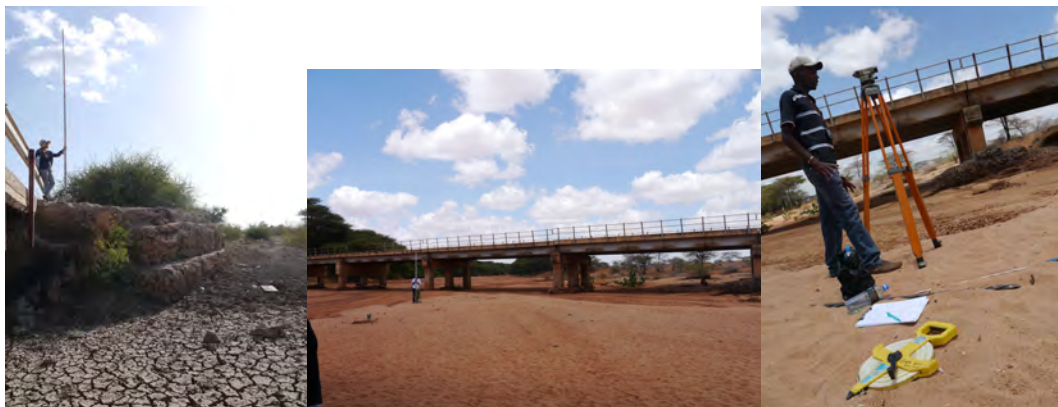
Figure 2.4: Fieldwork impressions: person holding staff (left), measuring elevation (middle) and sighting instrument (right)
