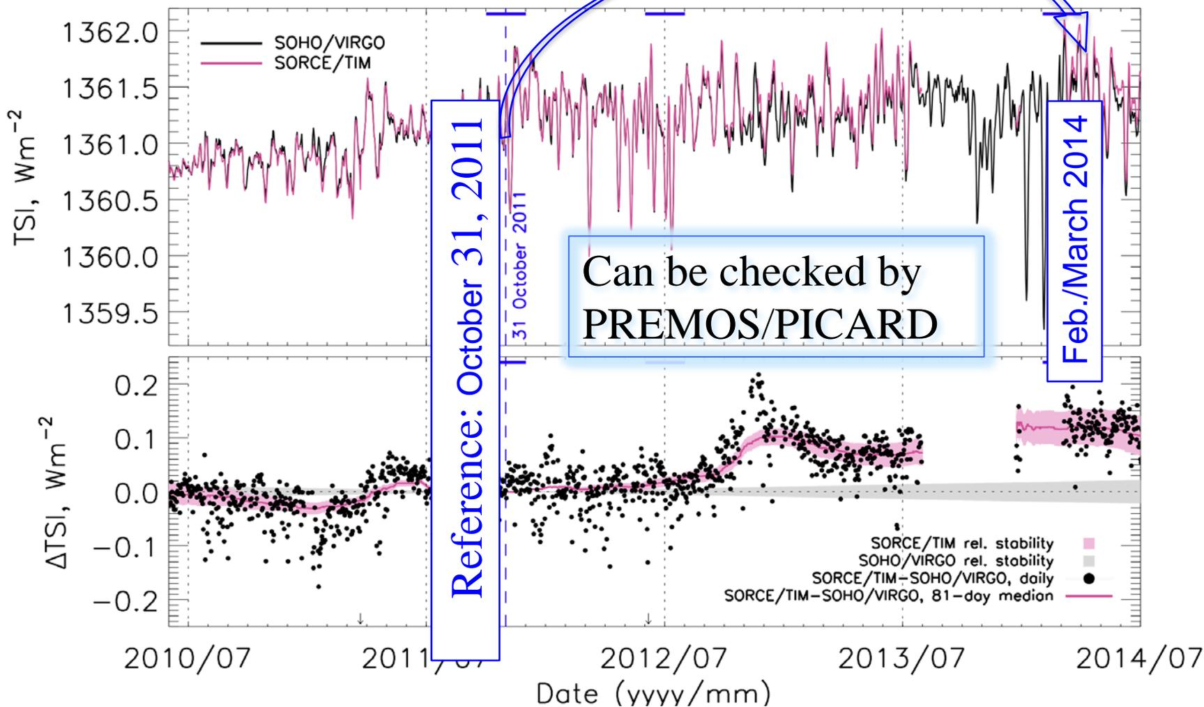
Standard tool to correct for inflight degradation:
