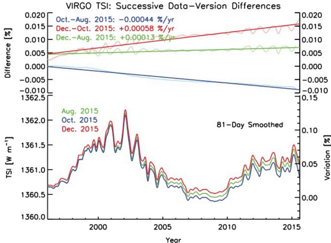
**Fig. 7.** Successive releases of VIRGO TSI data separated by 2 months each (lower plot) show significant trend differences (upper plot) due to variations in data-processing and estimates of instrument degradation with time.
