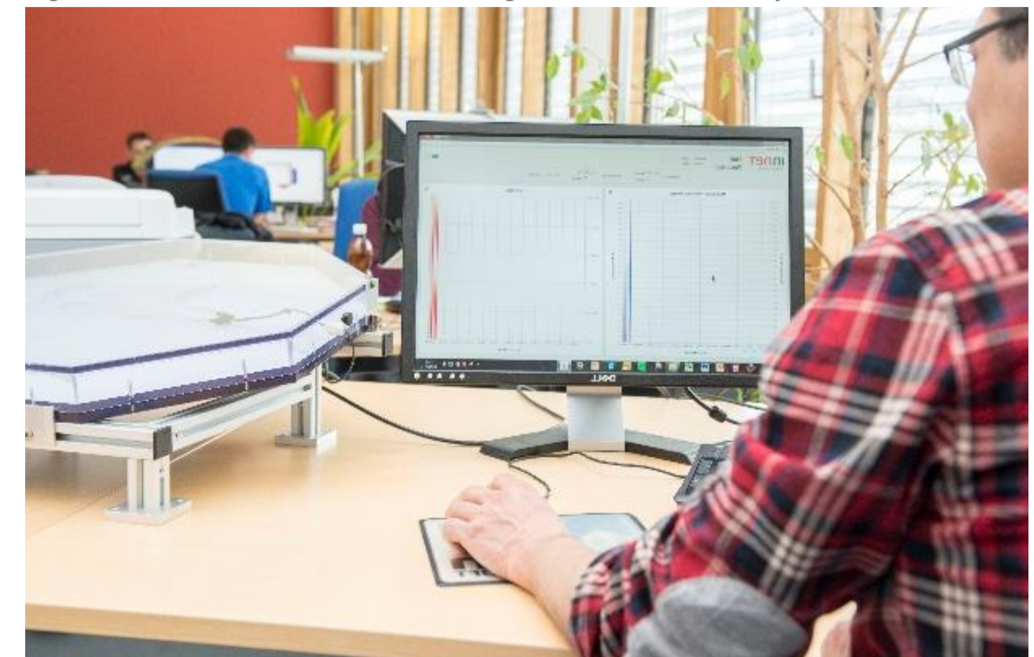
Figure 4: HailSens software suite collecting real-time Hailstorm dynamics data
